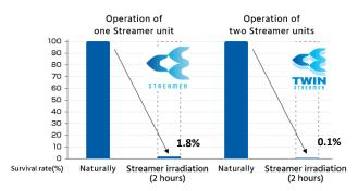
The survival rate of virus after 2 hours of Streamer irradiation was 0.1% for two units operation compared to 1.8% for one unit operation, confirming that the suppression effect was 18 times.
